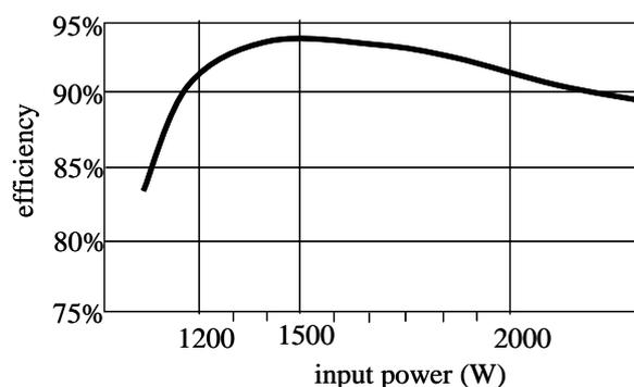
Figure 1. Inverter efficiency as a function input power
